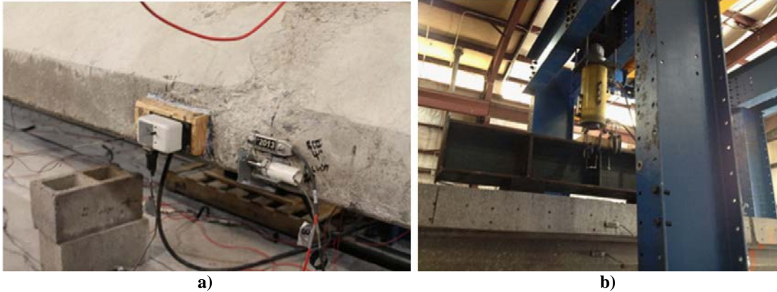
Figure 30. a) MLVDT, Strain Transducer, and Potentiometer and b) Load Cell, Actuator, Spreader Beam, Rubber Bearing Pads
