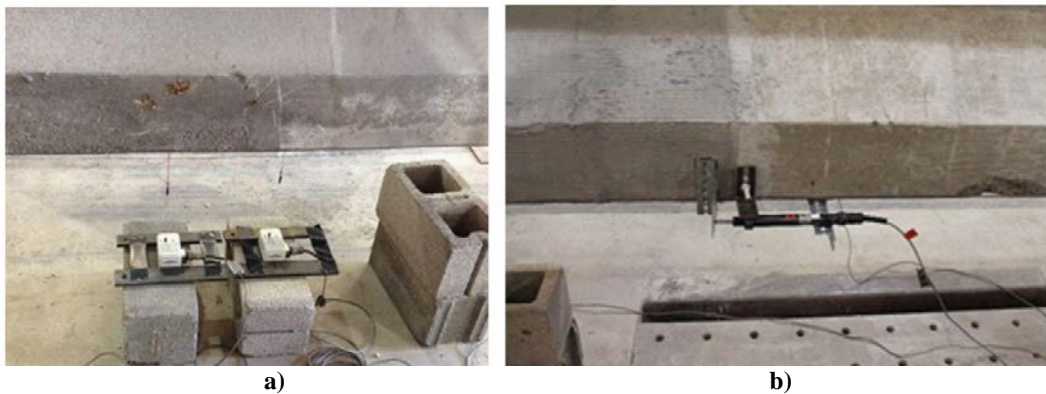
Figure 29. Measurement of a) Displacement using Wire Potentiometers Below Load Point and b) Slip Between Beam and FRCM Repair Material Using LVDT
