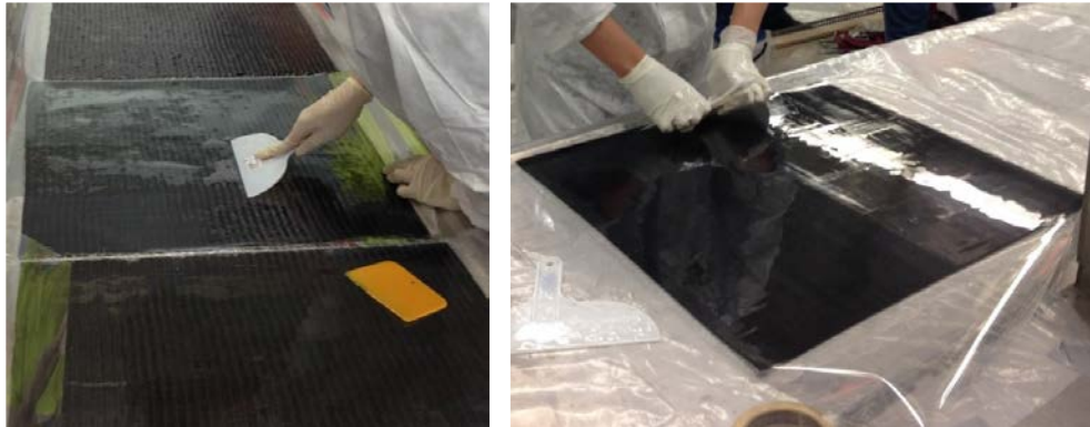
Figure 7. FRP Panel Fabrication
