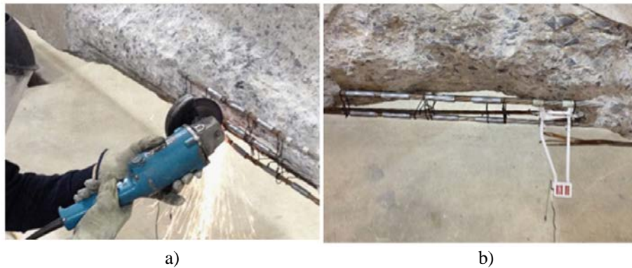
Figure 11. a) Electric Grinder Cutting a Strand, b) Extensometer to Measure Length Change
